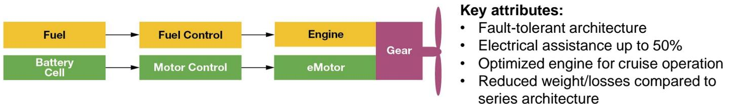
**Figure 4** – Project 804's hybrid-electric propulsion architecture.
