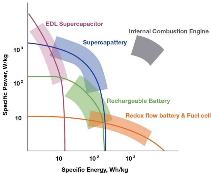
**Figure 2** – Ragone plot of energy storage technologies. Chen, George. (2017). (Open Access) Supercapacitor and supercapattery as emerging electrochemical energy stores. *International Materials Reviews*. 62. 173-202. 10.1080/09506608.2016.1240914.
