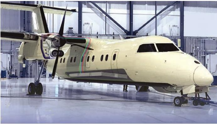
**L**everaging its breadth as an aerospace supplier, United Technologies Corp. (UTC) is modifying a Bombardier Dash 8 Q100 regional aircraft into a hybrid-electric flight demonstrator and may offer the conversion commercially after the X-plane flies in 2022. UTC is projecting energy savings of at least 30%.
